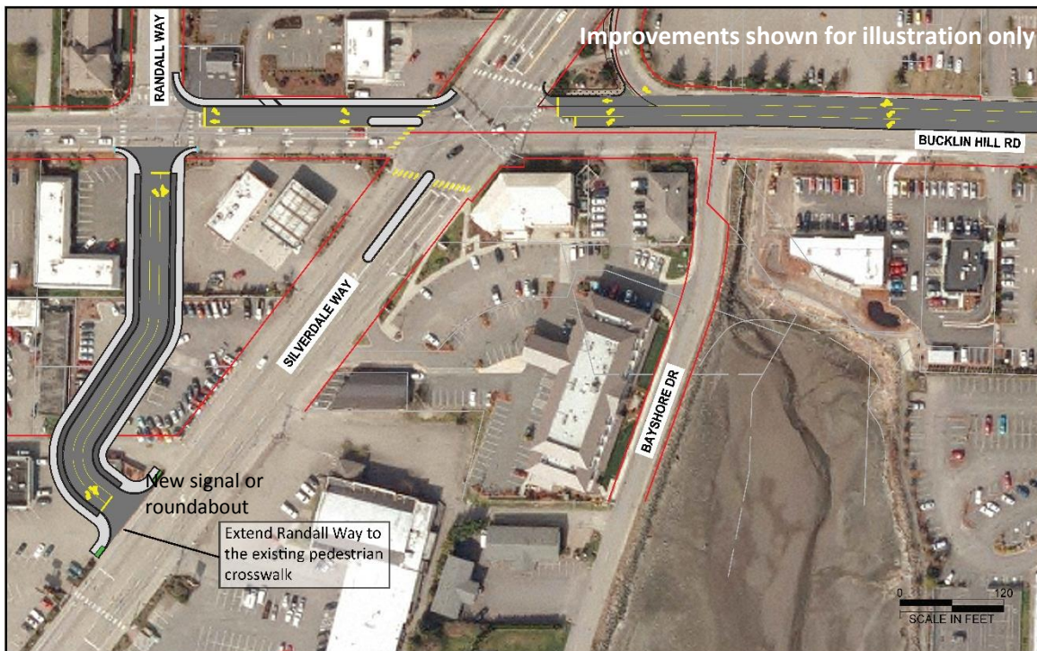
Figure 15. Randall Way Roadway Extension Options
