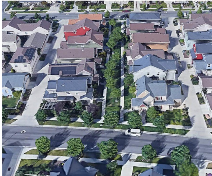
Figure 1. An example of a subdivision integrating alley access lots, which allows for the integration of open space corridors in place of some streets. Note that that the shallow garage driveways allow extra space for delivery trucks and on-street parking on the perpendicular streets helps to accommodate guest parking for these alley access lots.
