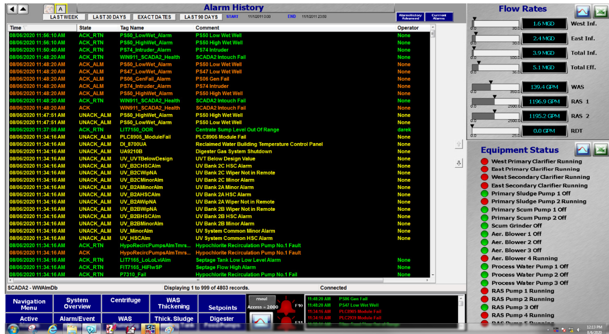
Figure 4-12. CKTP alarm history HMI screen
