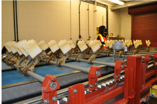
M-615 Gravity Belt Thickener
