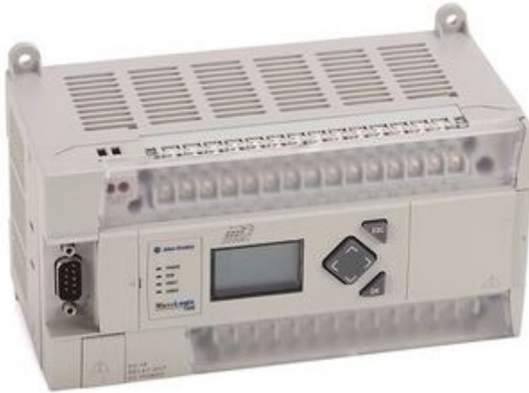
Figure 3-2. Allen-Bradley 1766-L32BXBA MicroLogix 1400 PLC
