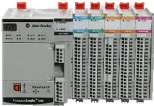
Figure 4-1. Allen-Bradley CompactLogix 5380 controller with Compact 5000 I/O modules
